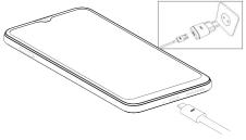
Use only General Mobile approved chargers, batteries, and Type-C cables. Unapproved chargers or cables can cause the battery to explode or damage the device. Connect the Type-C cable to the USB power adaptor and then plug the end of the Type-C cable into the multipurpose jack.
