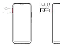
Only nano-SIM cards work with the device. Otherwise, device may be damaged.
