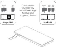
Only nano-SIM cards work with the device. Otherwise, device may be damaged.
