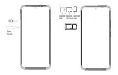
Only nano-SIM cards work with the device. Otherwise, device may be damaged.
